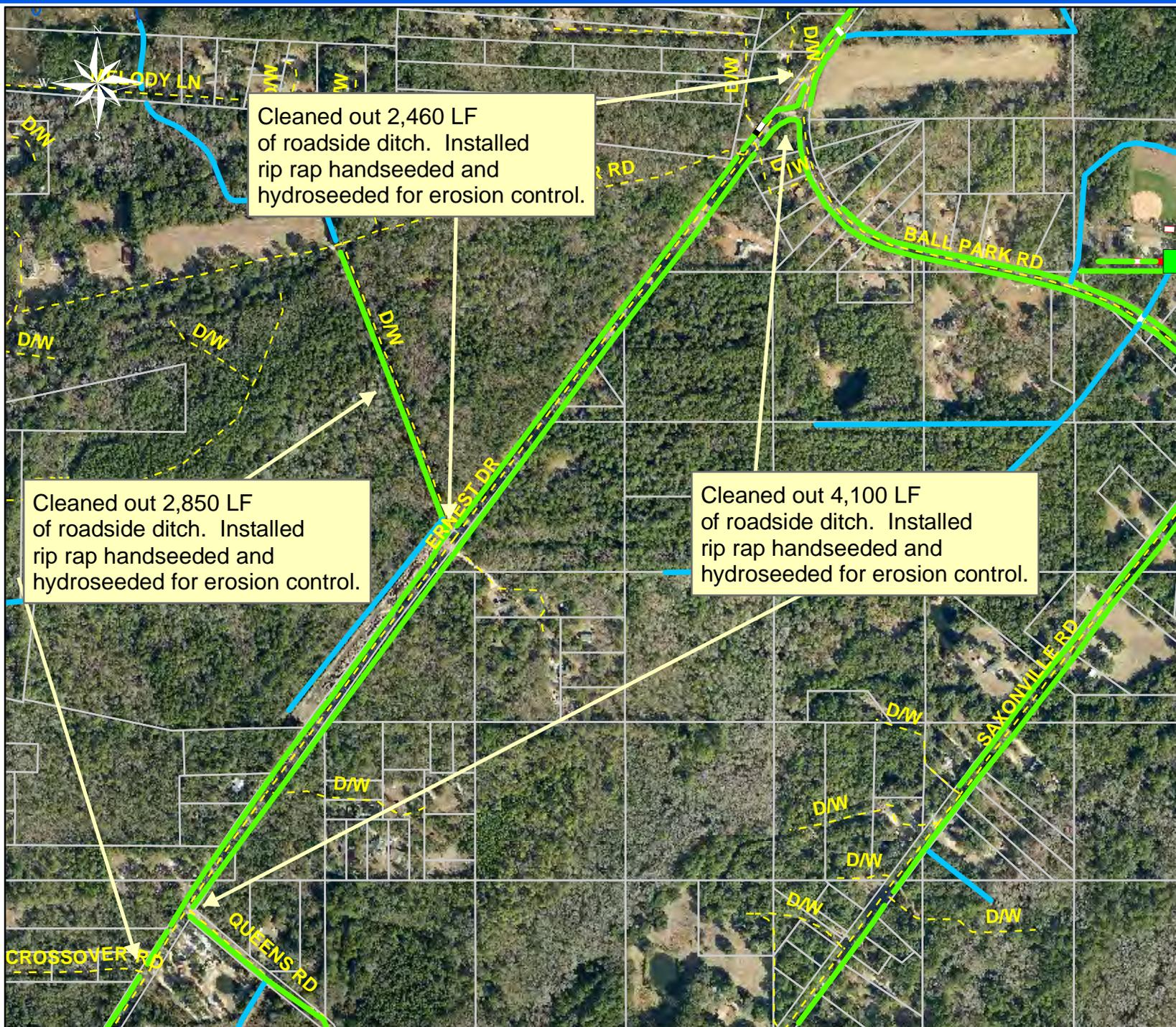
Cleaned out 2,460 LF of roadside ditch. Installed rip rap handseeded and hydroseeded for erosion control.
